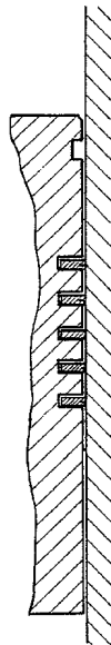
Figure 4.45 A large marine diesel engine piston with five piston rings. (Source: Patent WO 2004/090389)
