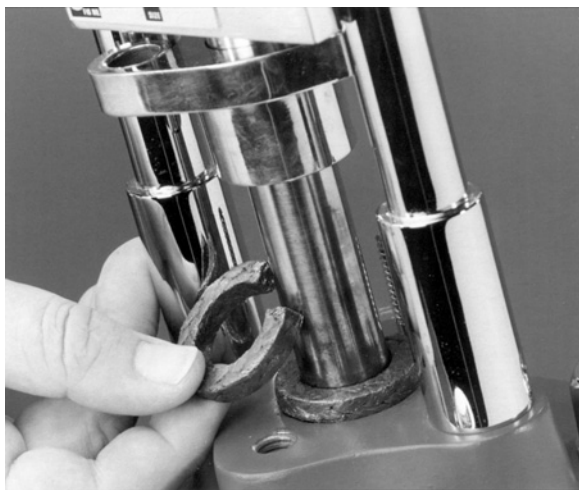
Figure 3.130 Photo of packing being fitted. (Source: James Walker)
