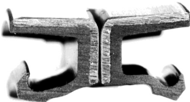
Figure 6.24 Seal distorted by use at excessive pressure, in this example 2 bar. Original profile is on the right. (Source: BHR Group)
