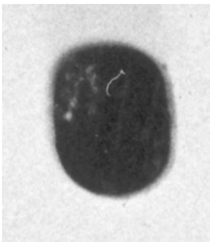
Figure 6.6 High compression set of a perfluoroelastomer O-ring when released at room temperature. It may continue to function at elevated temperature. (Source: BHR Group)
